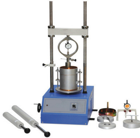
[ Figure 3.12 California Bearing Ratio CBR Apparatus, Source:Google ]
