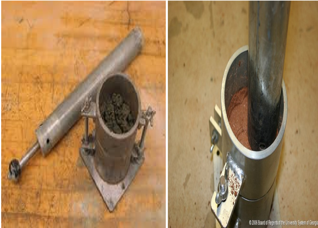
[ Figure 3.8 Proctor Compaction Test, Source:Google ]
