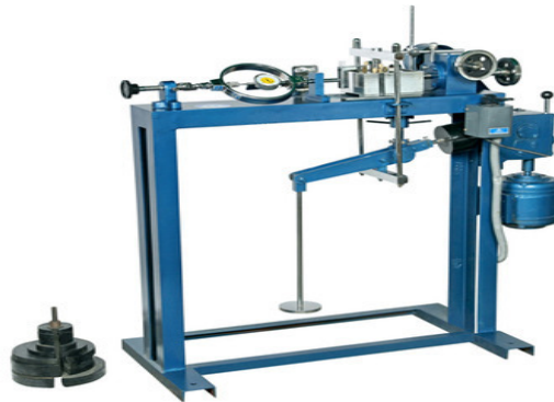
[ Figure 3.9 Direct Shear test Apparatus, Source:Google ]
