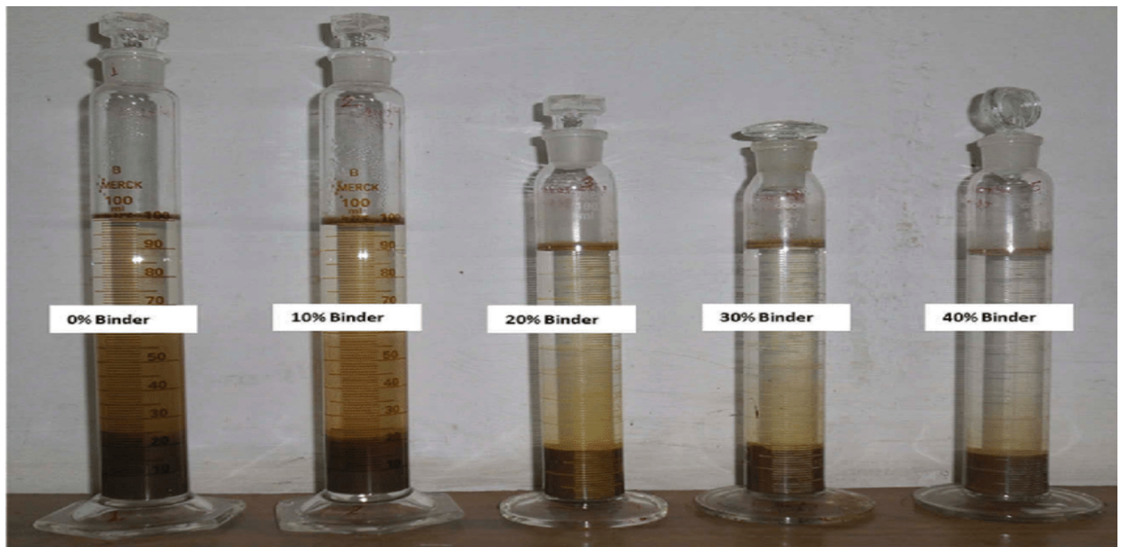
[ Figure 3.6 Free swell test for expansive soil , Source:Google]
